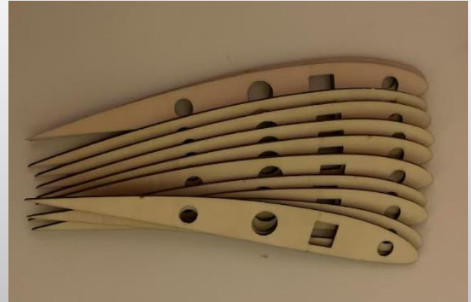
Figure 20: Balsa Wood Ribs Cut with a Laser Cutter
